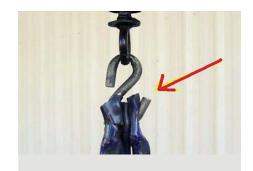
This photo is an example of an S hook that has not been completely squeezed closed.
