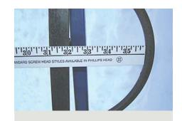
This photo is an example of a piece of playground equipment that has an opening larger than 3.5 inches and would pose an entrapment hazard.
